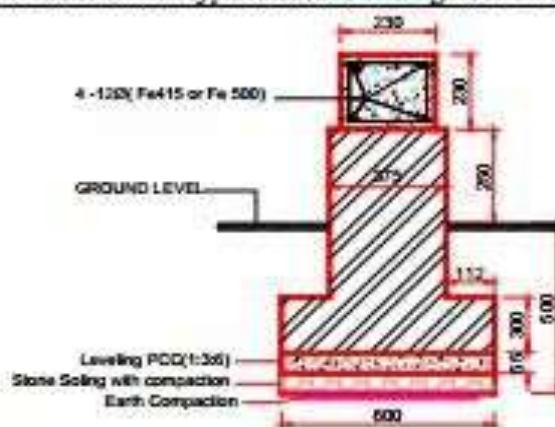
Figure (b) OPTION-II: Stone Masonry Toe Wall
